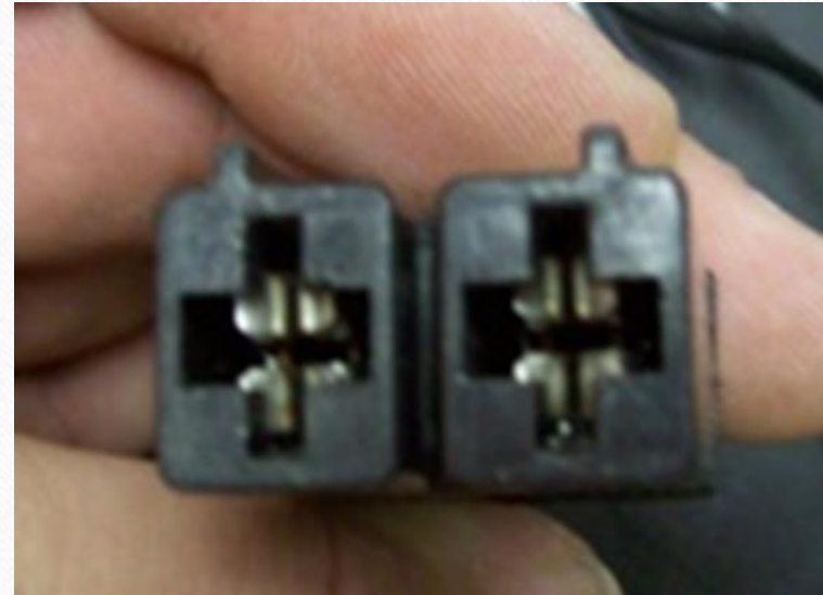
Q-Logic Power Connection Input to Power Module
