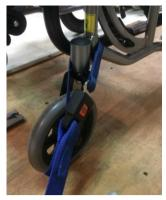
Fitting the Front Restraint
