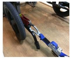
Fitting the Rear Restraint
