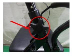
Insert push handles at least to the first cross hole into the frame tubing. Insert the fixing screw from the inside and tighten using the washer and star screw. To change the height adjustment of the push handles, loosen the fixing screw by turning the star screw counter-clockwise. Then lock the handle at the desired height, as described above.
