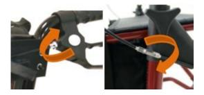
If the braking is poor or too hard, the brake can be adjusted either at the brake housing above or using the adjusting screw on the Bowden cable below) to achieve the desired braking effect.
