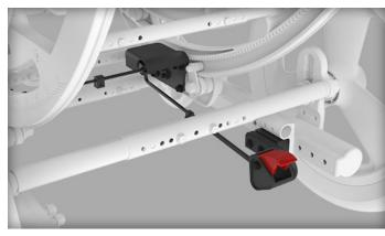
Can be ordered for either left or right mounting depending on preference. This option features a cable free mechanical linkage for the ultimate in low maintenance.
