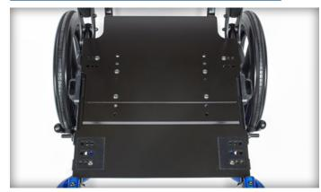
Grows 2" in width from even widths and 1" from odd widths. Depth growth is matched to Frame Depth Range and can be adjusted to any depth in the range: 14-18", 16-20", 18-22"
