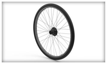
Hybrid wheel, hub design w/ straight pull radial spokes on the outside flange. Inside flange has a 2 cross spoke pattern to handle the torque resulting from stopping a larger wheel by the relatively small hub.
