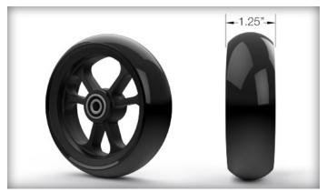
The wider profile uses molded polyurethane to create a great tyre. Hard on the outside for low rolling resistance, soft on the inside for cushioning. Available in 4", 5", 6", 7" and 8".
