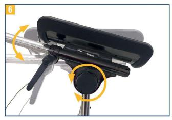
Gradually open the clamp screw on the side until you can move the forearm rest out of the locking position. Once you have adjusted the incline, move the forearm rest back into the locking position, then re-tighten the clamp screw.
