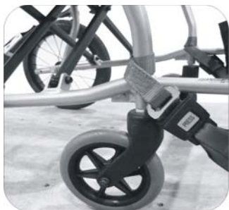
Fitting the front restraint
