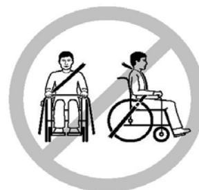
Incorrect seat belt position
