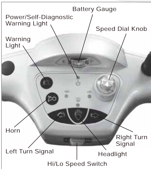
Figure 2 - HS-890 Control Panel
