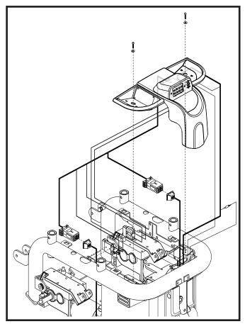
Figure 17. Jazzy 1121 Electronics Tray Assembly/ Disassembly
