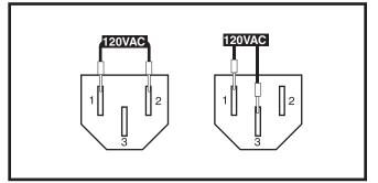
Figure 22. Charger Power Cord 3-pin Connector
