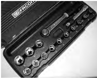
Flex ratchet and Socket wrench bits sizes 8 -19
