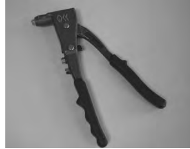
Pop rivet gun for rivets up to Ø 5 mm
