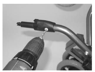
Replacing the Upper Swivelling Part of the Front Wheel Attachment
