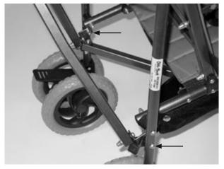
Next, loosen and remove the screw connections between the folding scissor construction and the posterior frame and remove the folding scissor construction.
