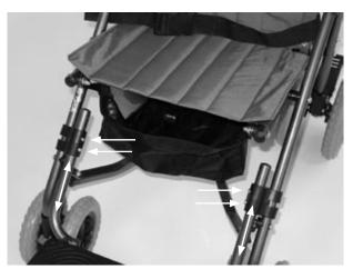
Replacing the Footrest Assembly - Adjusting the Lower Leg Length
