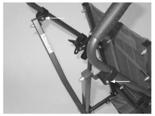
Replacing the Folding Scissor Construction for Back
