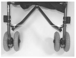
Loosen and remove the screw connections between the anterior frame and the folding scissor construction.
