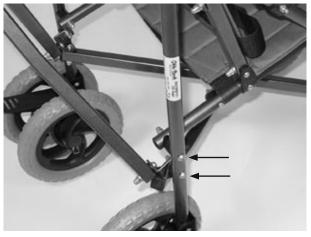
Next, loosen and remove the screw connections between the the posterior frame and the folding scissor constructions as well as between the posterior frame and the seat tubes.
