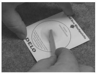
Open the two part adhesive sachet. Use the spatula to squeeze out all the contents of the sachet into the centre of the mixing card and mix the components for approx. 30 seconds.
