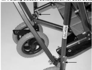
Replacing the Folding Scissor Construction for Seat Bottom
