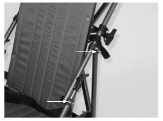
Next, loosen and remove the screw connections between the push handle and the posterior frame as well as between the push handle and the anterior frame.
