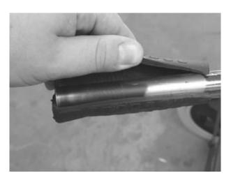
Carefully cut open the rubber hand grip using a stanley knife and remove the old rubber hand grip.
