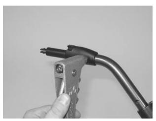
For re-assembly, plug all elements together and fasten the upper swivelling part using two rivets.
