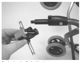
**Replacing the Swivel Lock**
