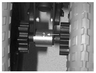
With a few models, the rear axle is additionally fixed with a set screw. Loosen this set screw and then pull the axle out of the rear wheel attachment.
