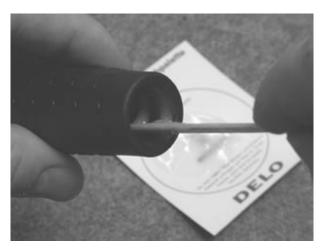
Apply half of the adhesive into the rubber hand grip using the spatula. Evenly distribute the adhesive in the rubber hand grip up to a depth of approx. 4-5 cm.
