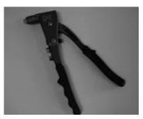
Pop rivet gun for rivets up to Ø 5mm
