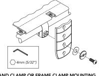
BAND CLAMP OR FRAME CLAMP MOUNTING (Requires Art. No. HW320 or HW310) Attach clamp to seat tube. Attach belt using the M6 screw included with the clamp.
