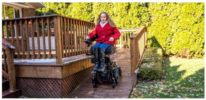
A powerchair's capability to drive up slopes can be impacted by the user weight, speed and the powerchair setup. Manufacturers therefore provide a maximum slope of incline that each powerchair can safely ascend or descend and we recommend users do not exceed the maximum allowable incline listed in the chart below:
