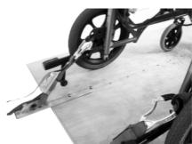
Fitting the rear restraint
