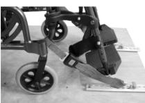
Fitting the front restraint
