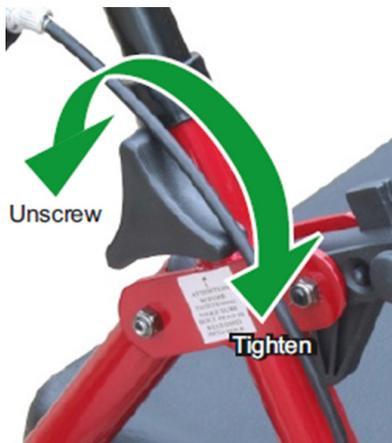
To adjust the height of the handlebars, unscrew the tightening handles on either side of the Rollator turning anti-clockwise and remove. Adjust the height of the handlebars to suit the user, re-insert the tightening handles and tighten by turning clockwise to secure (as shown in the picture). Ensure that the tightening handles and brake cables are on the outside of the Rollator.
