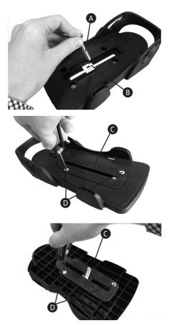
Insert the required attachment bolt along with the retention plate **B**. Place a rubber lid **G** on, both, the top and bottom of the sandal. Fasten using the four screws **D**provided. To remove or replace the attachment bolt, reverse this process.
